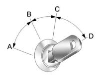
The ignition switch has four different positions.
